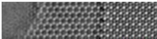
Figure 5. TEM image of single-layer and double-layer graphene [7].
