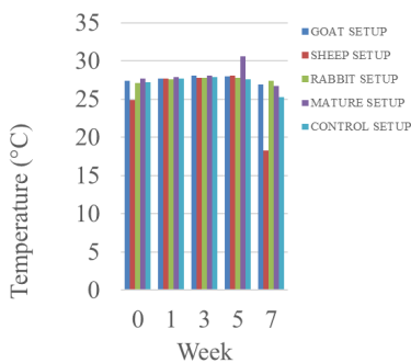
Figure 7. Gradual development in the temperature (Temp) (°C) during composting.
